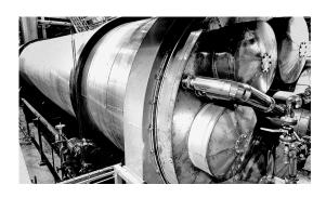
The Haarslev Tube Bundle Dryer is a compact steam dryer for the drying of biomass (sawdust, peat) and various protein-based feedstuffs such as fish meal and distiller's spent grains (DDG and DDGS) providing high evaporating capacity and consistent product quality.
